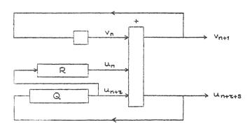
Here Q and R denote delay lines with length q = s-r > 0 and r respective-ly. We have
