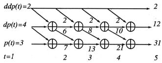
The method computes the values of the polynomial for each location in the range using a mere *n* additions per location. This implies that decomposing a shading function in a vertical component and a horizontal component which is constant per scanline, both of which can be expressed as polynomials only, would produce a very efficient shading technique.
