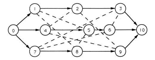
Figure 1: Disjunctive graph for a 3-job 3-machine problem
