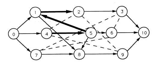
Figure 2: Disjunctive graph after sequencing machine 1
