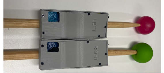
(a) RemixDrum 3.0 equipped with haptic feedback and real-time position tracking via colored spheres.
