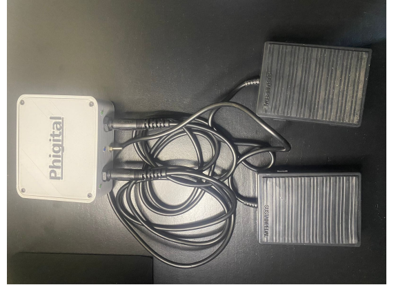
(b) Electronic foot pedals used for triggering virtual drum components. The pedals are connected to a circuit that transmits activation signals to the application via OSC.
