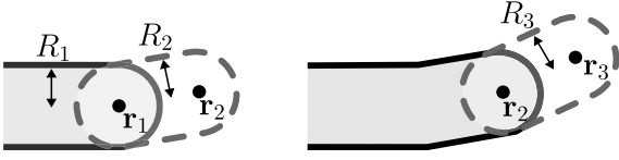
Fig. 2. Illustration of how cylindrical segments with a semi-spherical cap can be added together to extend a channel from \mathbf{r}_1 to \mathbf{r}_2 (left) and afterwards from \mathbf{r}_2 to \mathbf{r}_3 (right). We assume a constant radius R along an individual segment. Note that the respective \mathbf{r} coordinates are defined at the ‘center’ of the segment’s caps. The figure is not to scale: in actual simulations, the length of a newly added segment is comparable to the streamer radius or smaller, see section 4.3.
