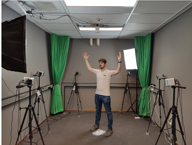
Figure 5.1: Physical camera arrangement from the CWIPC-SXR dataset
