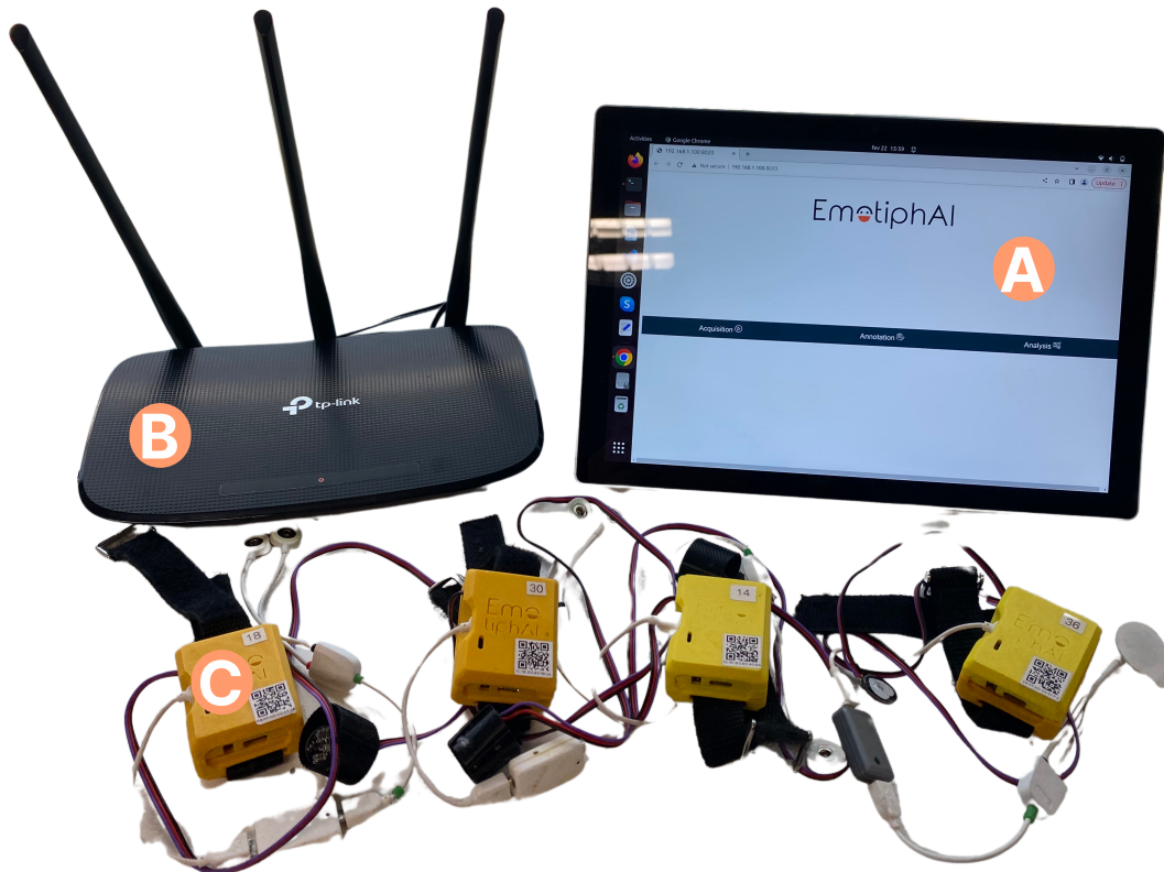
Figure 7.2: EmotiphAI platform setup used in the Differential cinema sessions. Nomenclature: EmotiphAI Collector (A); TL-WR940N router (B); EmotiphAI Wearable based on the ScientISST device (C).
