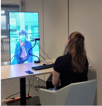
Figure 5.3: Static AR system without perspective projection. A 3D sensor captures the user in photorealistic representation.
