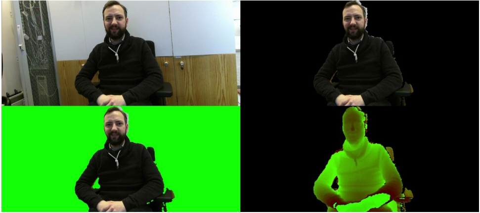
Figure 5.2: Different Video Capture modes A (top left) full color, B (bottom left) green-screen cut-out and C (right) color cut-out (top) with depth (bottom).
