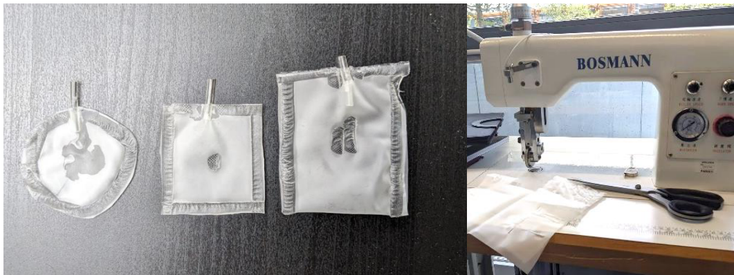
Figure 42: Ultrasonic sewing on PE-film to create airtight airbags (left), airbags produced (right).
