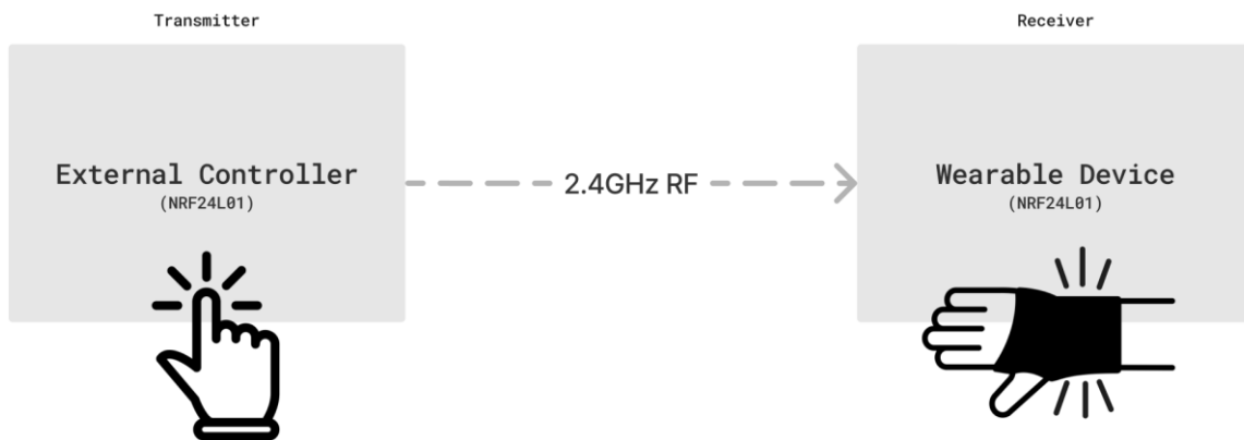
Figure 46: Schematic of data connection between the wireless controller and wearable device.
