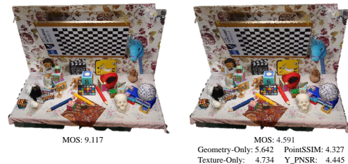
Figure 3: Point cloud Unicorn comparison between learning-based and traditional FR metrics. The left side shows the reference Unicorn, while the right side displays the distorted version with geometry Gaussian noise (points randomly shifted within 0.02%).
