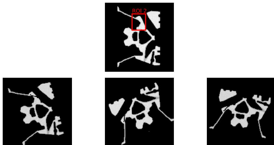
Figure 7. The top row depicts the selected ROI from the initial dataset, devoid of any defects. The bottom row presents three samples with artificially inserted crack defects within the ROI, each sample exhibiting a unique combination of rotation and scale variations to simulate defect diversity.
