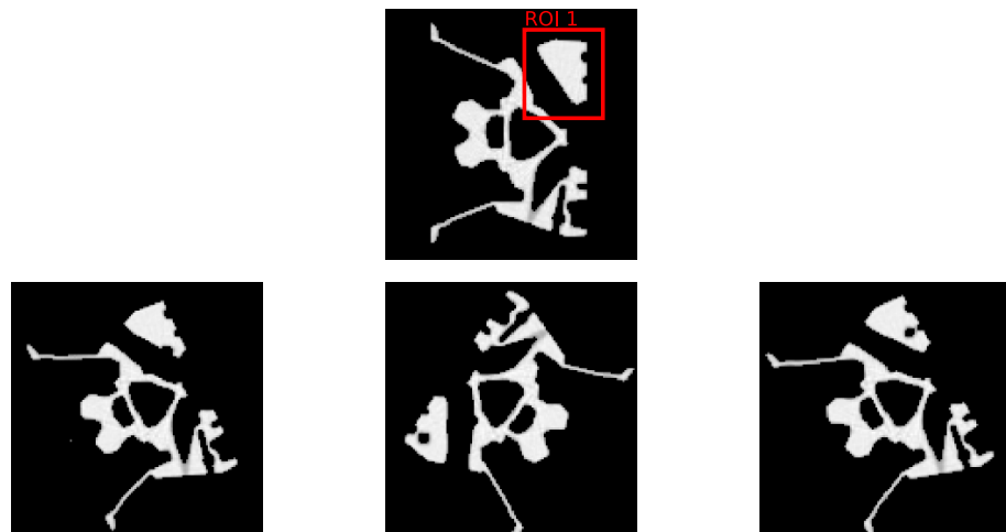
Figure 6. The top row depicts the selected ROI from the initial dataset, devoid of any defects. The bottom row presents three samples with artificially inserted pore defects within the ROI, each sample exhibiting a unique combination of rotation and scale variations to simulate defect diversity.
