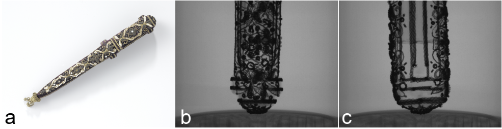
Figure 1.6: a) Cutlery case from the Rijksmuseum collection [158], b) and c) two radiographs of the lid of the cutlery case, with c) rotated ninety degrees with respect to b). Image adapted from [106].
