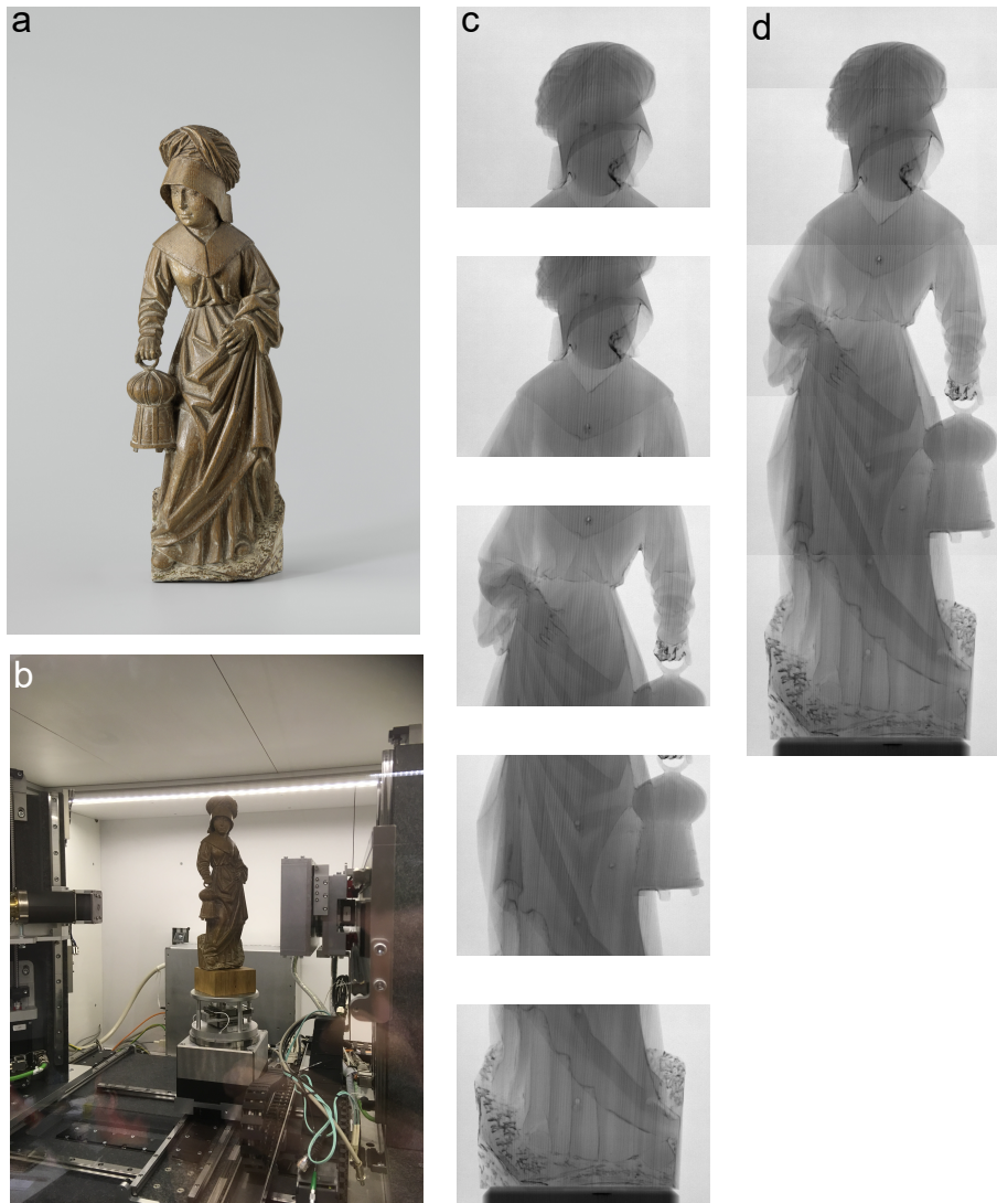
Figure 2.6: Example CT scan of a wooden sculpture to illustrate tiled scanning. a) Woman with lantern [159]. b) The sculpture mounted on the rotation stage in the FleX-ray scanner. c) Radiographs showing the five tiles needed to image the entire object. d) The radiographs in (c) combined to obtain a single radiograph of the entire sculpture.
