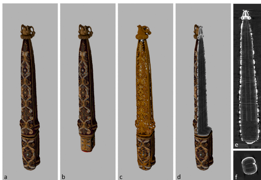
Fig. 8. a) Surface scan of the cutlery case and lid - aligned using the CT of the full object, b) surface scan of the case only, c) CT volume representation and surface scan of lid, d) surface scan, cut open to show the CT slices, e) corresponding vertical slice, f) corresponding horizontal slice.
