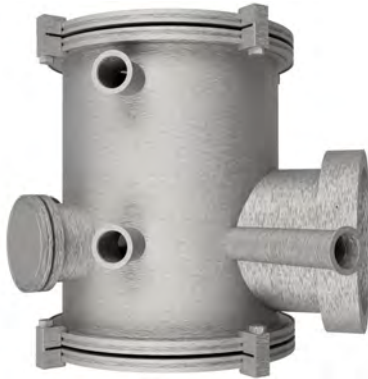
Figure 3.17: The geometry of the experimental discharge vessel, as seen from the side. It is a quasi-cylindrical vessel that contains observation windows and gas flow tubes. The ICCD camera captures pictures through the large window on the right. We observed that streamers propagated slightly off-axis, with the deviation towards the largest window, which is most likely related to the electric potential distribution inside the vessel.
