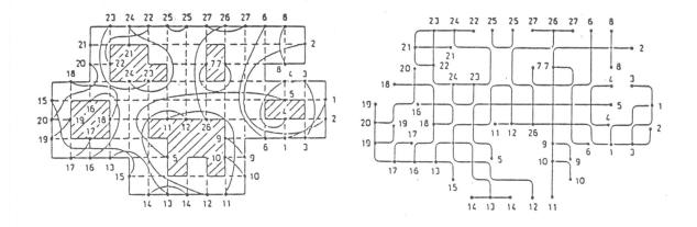
Fig 1. A Local Routing Problem and its solution. The global routings are shown as curves for added clarity.
