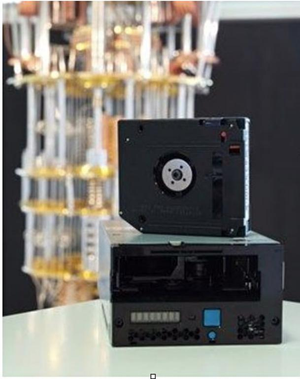
The company said it has tested CRYSTALS successfully on a prototype IBM TS1160 tape drive using both Kyber and Dilithium in combination with symmetric AES-256 encryption, enabling what it calls the world's first quantum computing-safe tape drive.
