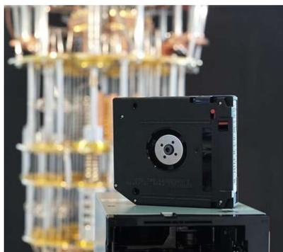
The new IBM quantum computing-safe tape drive prototype is based on a state of the art IBM TS1160 tape drive. Credit: IBM
