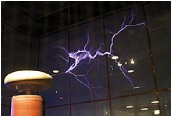
Figure 1.1: Tesla coil demonstrating electrical breakdown process.
