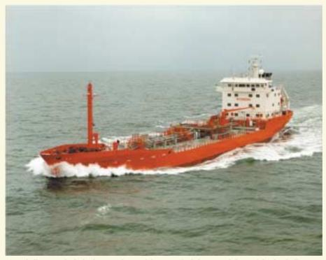
One challenge in the hydrodynamic design of ships is to find the optimal shape of the ship hull satisfying prior requirements of use, economy, safety, etc. CFD computations have led to improvements of the hull shape, so that the high amplitude of the long waves made by the ship could be strongly reduced. (Photo courtesy MARIN.)
