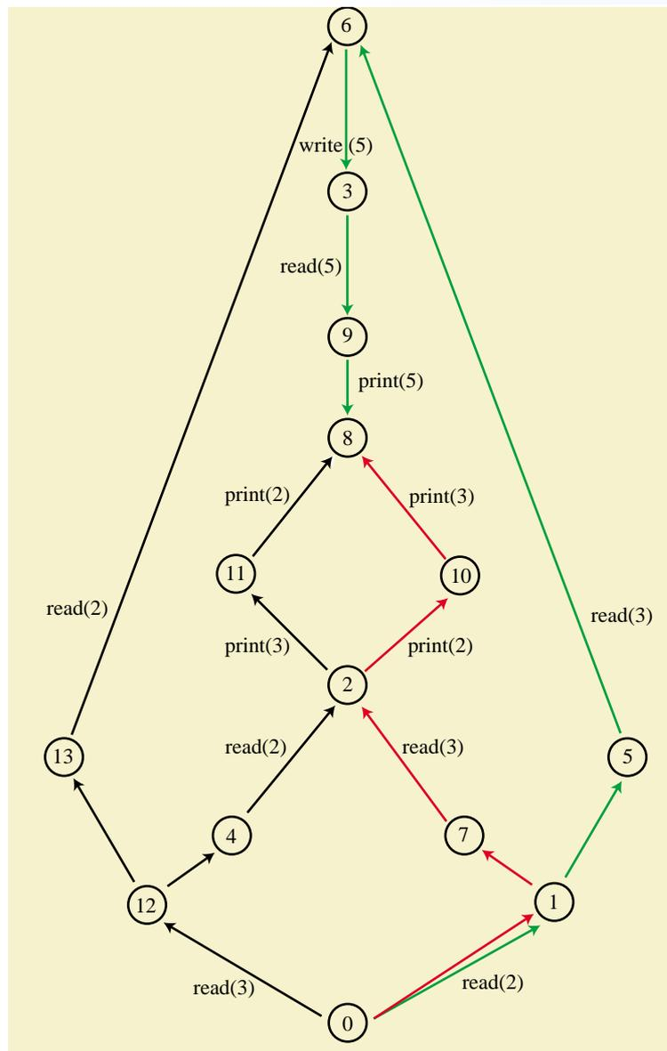
Figure 3: A correct path (green) and a wrong path (red) of the system with two adders on the set {2, 3}. Starting state: 0. Final state: 8.
