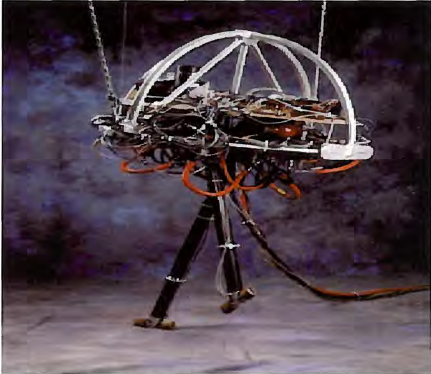
Figure 1. The 3D Biped robot, developed at MIT, hops, runs and performs tucked somersaults. (Courtesy MIT Leg Laboratory.)
