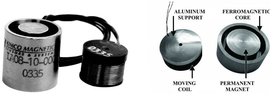
Figure 6.1: A cylindrical voice-coil actuator consisting of a ferromagnetic core, permanent magnet and coil.
